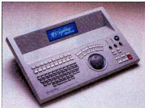
The 360 Systems Shortcut redefines the low end of proprietary DAW systems. Using an internal hard drive, the 2-in/2-out unit offers simple and fast editing of stereo audio on dedicated controls.
